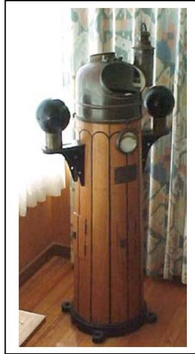
The original binnacle that was mounted on the outer deck of the bridge. This was used in conjunction with the external steering position.
