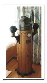
The original binnacle that was mounted on the outer deck of the bridge. This was used in conjunction with the external steering position.
